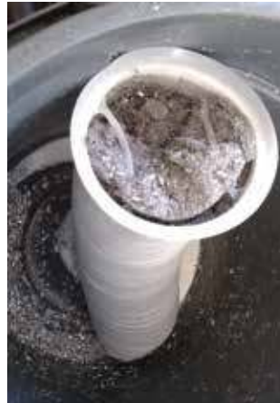
Filter bag full of aluminum fines removed from the filter housing.
