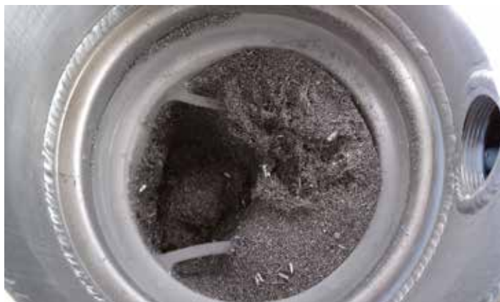
Aluminum fines fill the filter bag.
