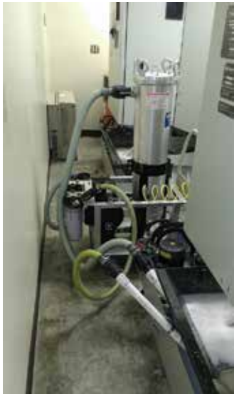
Pump/filter unit cleaning machine sump. (Model shown with optional cartridge filters on pump discharge.)
