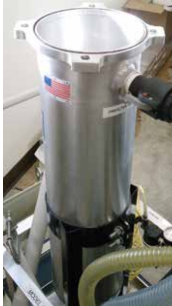
Pump/filter unit open for service.
