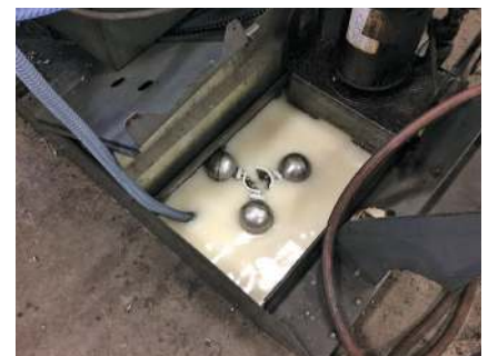
RSM-3 Floating Inlet Device (8" wide x 8" long)
