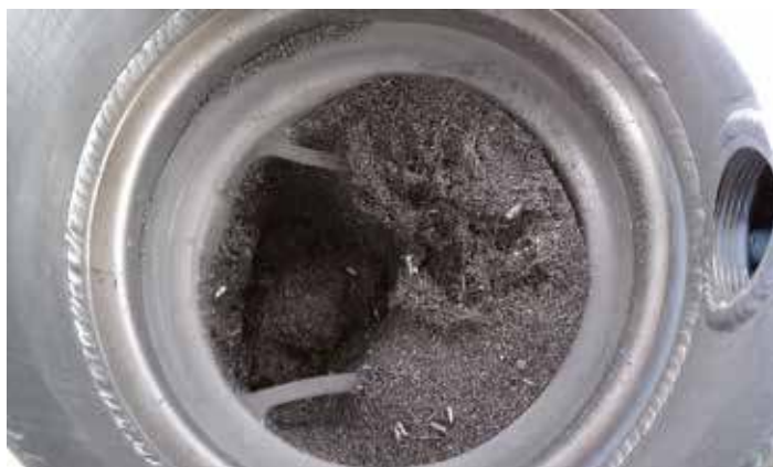
Aluminum fines fill the filter bag.
